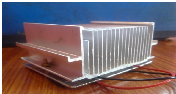
Fig 1. Thermoelectric power generator with fin
